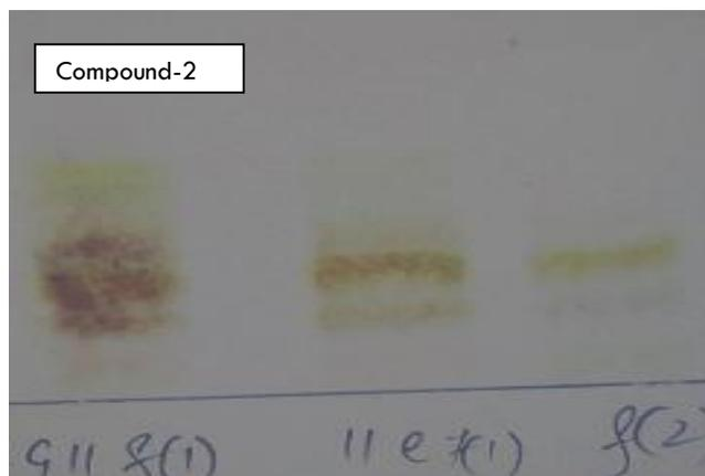
Figure 2: TLC chromatogram of fractions collected from column VII showing distinct spot of compound-2 (f2)
