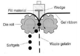
Figure 7: Mechanism of soft gel formation
