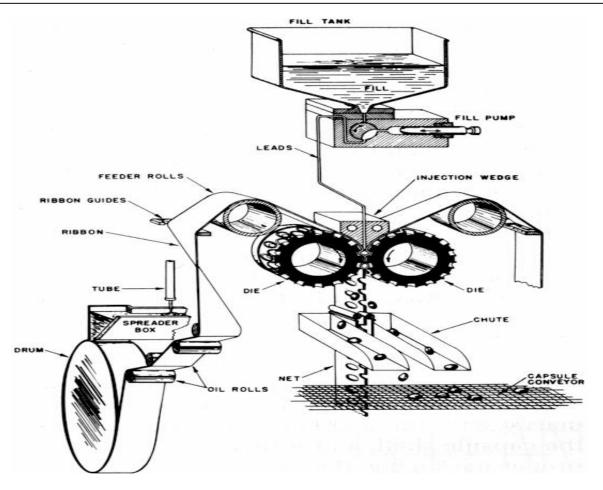
Figure 6: Schematic drawing of a rotary-die soft gelatin capsule filler (R.P. Scherer: Detroit, MI).
